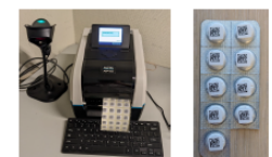
Picture 3: Stand-alone barcode duplicator By scanning the FMD-code in the original package, duplicator 2D barcodes are generated and printed. FMD-codes include article number (STIN), expiration date, serial number (for FMD) and lot number.
